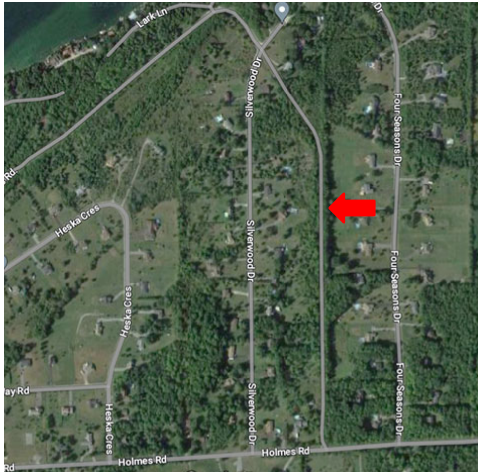
Figure 1. Image with right of way appearing as an unmarked road parallel to Silverwood Drive. 3
